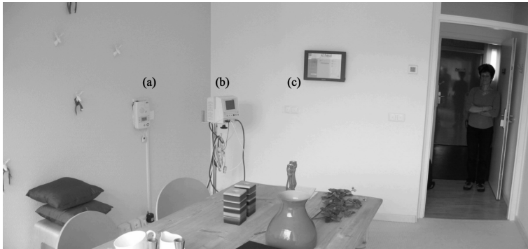
Fig. 1. Demonstration room with smart home technology: (a) Alarm unit; (b) Telemedicine monitoring system; (c) Touch screen with electronic patient file
