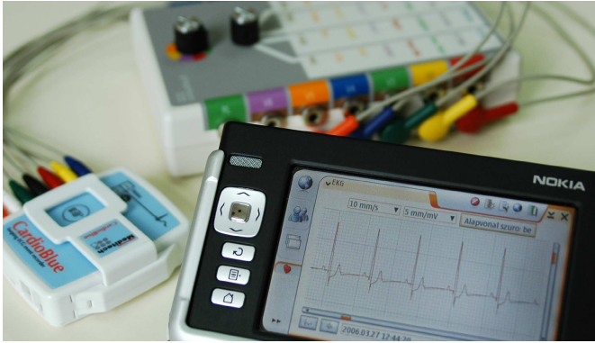
Fig. 1. The system setup: A Nokia Internet Tablet, a CardioBlue mobile ECG device, and an “artificial patient”
