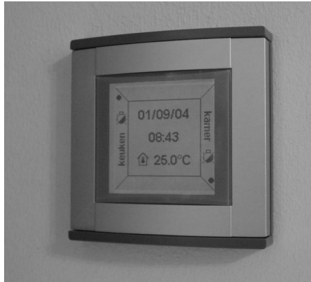
Fig. 2. The room controller allows you to control lighting, room temperature, and television, for example. This room controller is negatively evaluated by both care receivers and caregivers, mainly due to poor legibility [15].
