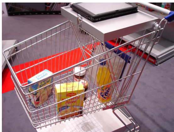
Fig. 1. BERNIE as a shopping cart equipped with an RFID-antenna, a laptop and a RFID-reader that is hidden beneath the cover plate
